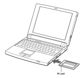
Do not force a card into the slot. It may damage the connector pins.
