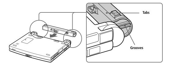
Slide the lock lever into the LOCK position to secure the battery on the computer.
