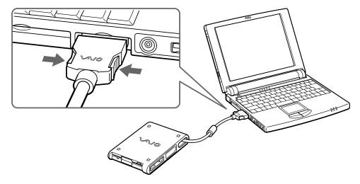
Fold the floppy disk drive cable into the compartment on the side of the floppy disk drive.
