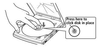
Be sure to seat the CD-ROM disc firmly over the CD-ROM drive hub fingers. If you do not seat the disc firmly, you could damage your CD-ROM drive.
